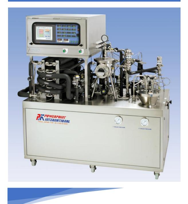
Designed for comparisons of heat treatment with either direct heating or indirect heating. The machine can be supplied with tubes, plates or both. Processing using either direct heating or indirect heating at temperatures to 152 deg C and flow rates from 10 to 40 Ltr per hour. Easy changeover from direct heating or indirect heating by the touch of a button. Just select which system is to be used from the touch panel menu and the machine is ready to use.
