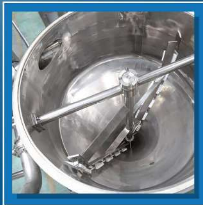
Inside Anchor Mixer of PVC-500 Mixer
