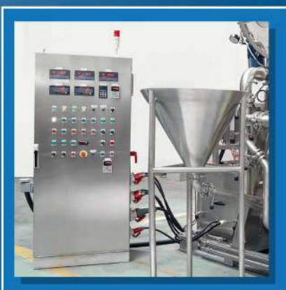
Pushbutton Electric Control of PVC Mixer
