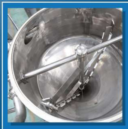
Inside Anchor Mixer of PVC-500 Mixer
