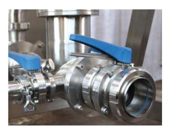
The inline mixer has several inlet ports, and the main inlet is connected with the bottom discharge of the tank, with other two inlets connected with other liquid and powder tanks. The inline mixer's outlet goes back to the top section of the mixing tank.
