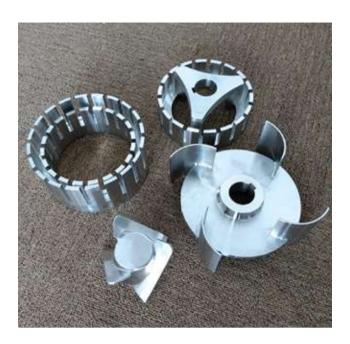
The basis of this plan is the PerMix innovative inline mixer, which has a mixing, dispersing and emulsifying head with multi-working chambers. It can be supplied with mixing vanes, dispersion components or emulsifying tools. For each operation, these components can be interchanged or combined so that the mixer operates to suit every product possibility.
