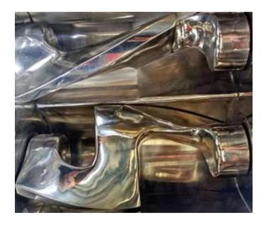
The mixing action is a combination of bulk movement, smearing, stretching, folding, dividing, and recombining as the material is pulled and squeezed against blades, saddle, and side walls. Continually new layers of material are compressed and folded over one another and are subjected to shearing forces. New surfaces are formed and the components can penetrate.
