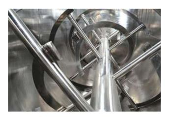
The shaft is sealed with stuffing box with multiple PTFE packings (sometimes with a lantern ring for air purge) at both ends. Materials are loaded from top side, and a flush fitting discharge valve is located at the bottom side in the center. The discharge height can be adjusted as per requirement, so that material gets discharged into the container below it without floating dust.
