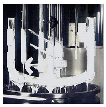
During operation of the PerMix PMS series Multi-shaft Mixer, the high speed blade provides high shear to disperse the materials, while the low speed blade keeps feeding the high speed blade by scraping material mass from near the wall.
