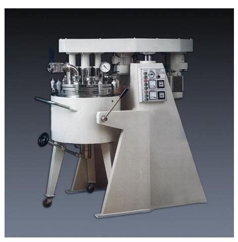
The PerMix PMS series Multi-shaft Mixer is a revolutionary universal multi-processing mixer which is designed to serve a wide variety of industries in many different processes. It provides a unique three-way mixing action by combining slowly running elements with a rapidly running element.
