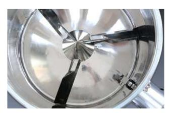
The PerMix PDI series High Speed Mixer, also called Mixer Granulator, Wet Granulator, or High Shear Mixer Granulator, is an efficient and versatile blending machine for mixing of dry powders, or granulating with the addition of liquid binder, within a very short time and with excellent cleaning abilities. It is able to give perfect result for mixing due to the innovative design of a central Impeller type mixer with a side vertical Chopper.
